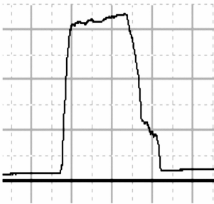
(c) 正间断负连续脉冲电流 (c) Pulse-reverse current without gaps in negative current
